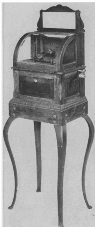
Figure 8, below: The Edison one-cent juke dates from 1887. The directions read, "Turn crank on side of cabinet eight times and let go, then drop one cent in slot."
